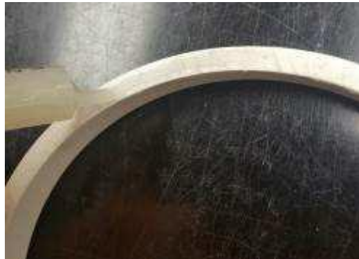
Figure 5 – Example application of Sealant to Bottom of Plastic Ring
