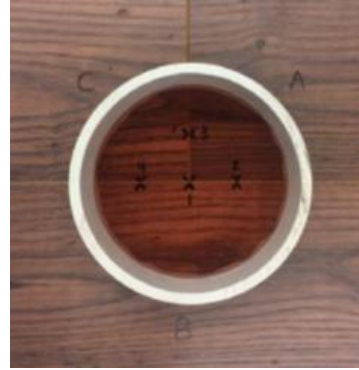
Figure 8 – Assembled Plank Surface Water Exposure Test Set Up
