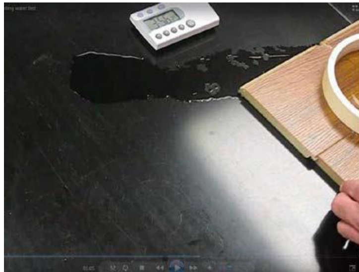
Figure 9 – Example of Joint Failure – Water Through Leakage
