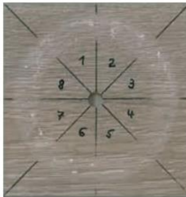
b) Correct test: Wear-through of more than 1,00 mm 2 is not obtained in octants 4 and 5
