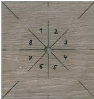
a) Insufficient test: Wear-through with an area of at least 1,00 mm 2 is only evident in octant 6 and 7
